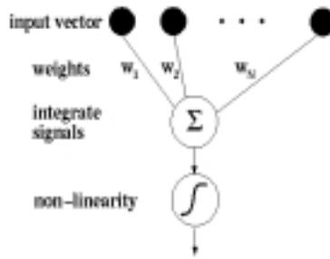
Figure 1: **Simulated neural units.** Artificial neural units take on a variety of forms, however, the general scheme is shown here. A neural unit collects information from other neural units along connections (synapses). Each connection is associated with a weight ( $w_1, w_2, \dots, w_N$ ) that can be changed according to preset rules. The unit typically has some integration step (here shown as a summation) and some kind of non-linearity before producing an output.
